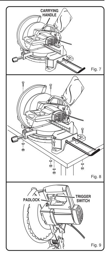
■ Install a padlock through the hole in the trigger switch.
